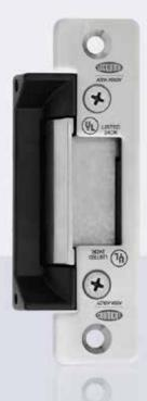
The Lockwood Padde Series ES110 is a cost efficient robust electric strike with a solid construction of one-piece cast aluminium body and stainless steel striker. Having a deeper than normal strike-keeper area, ES110 is designed to work with an extensive range of locks and offers the same level of security and reliability usually provided by more expensive electric locking solutions.
